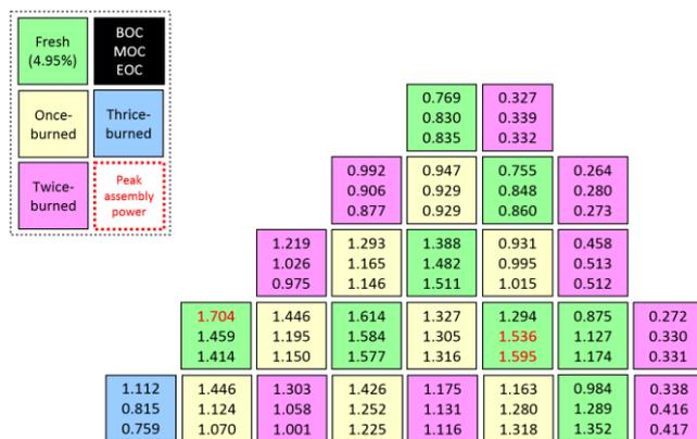
Figure 7. Normalized radial assembly power profile of 1/8th of the equilibrium SBF AP1000 core.
