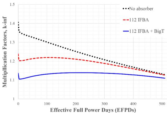
Figure 3: Burnup-dependent reactivity of the BigT- and IFBA-loaded fuel assembly.
