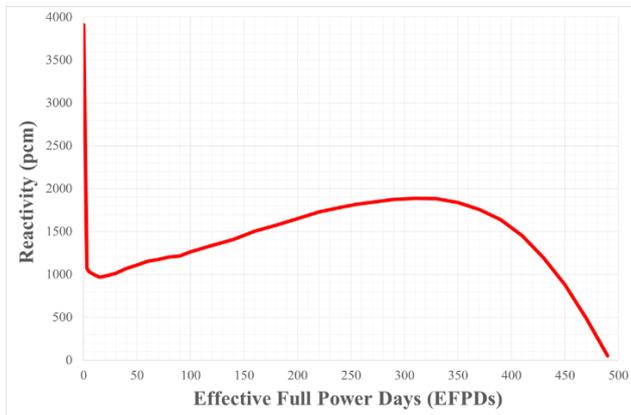
Figure 6. Reactivity depletion over equilibrium cycle of the SBF AP1000 core.
