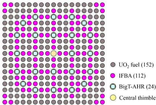
Figure 2: BigT- and IFBA-loaded fuel assembly.
