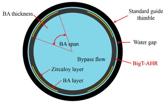
Figure 1: Design concept of the BigT absorber.
