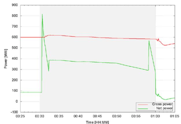
Figure 2: Gross and net power of the plant.
