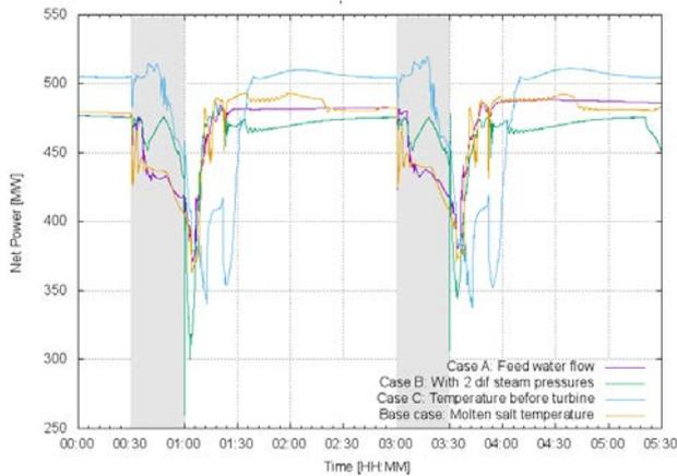
Figure 4: Net power production with different feed water control methods.
