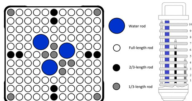
Figure 1: **TRITON11** fuel lattice cross-section geometry (left). **TRITON11** fuel bundle geometry (right).
