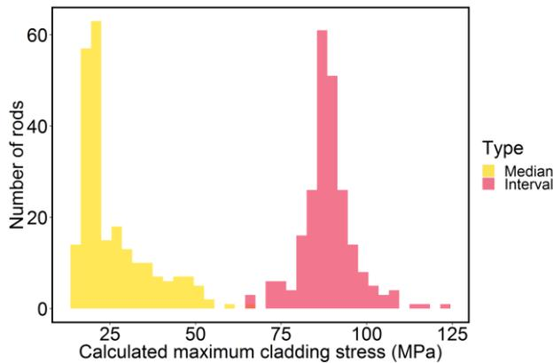
Figure 4: Uncertainty analysis results regarding maximum calculated cladding hoop stress. Notation as in figure 1.
