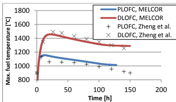
Figure 2: Comparison of maximum fuel temperatures during D/PLOFC accidents in HTR-PM [3].
