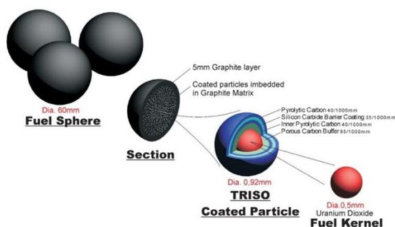
Figure 1: Schematic of a pebble bed reactor fuel.
