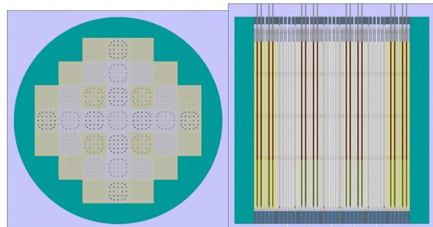
Figure 1: Horizontal and vertical plots of the modelled core geometry Serpent model. The plots show the regulating bank inserted into the core and the shutdown bank extracted.
