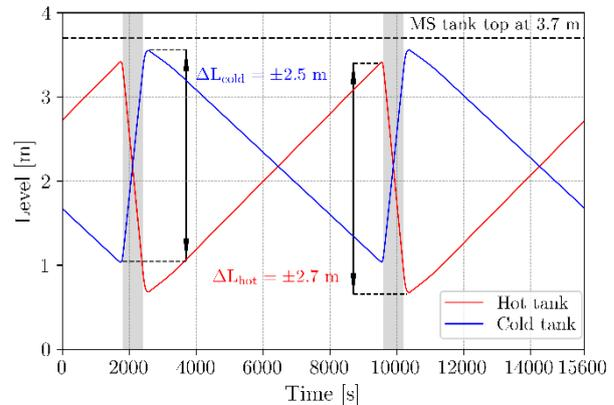
Figure 4.2 Cold and hot salt storage tank levels in the small ESS of the HCPB plant [2].
