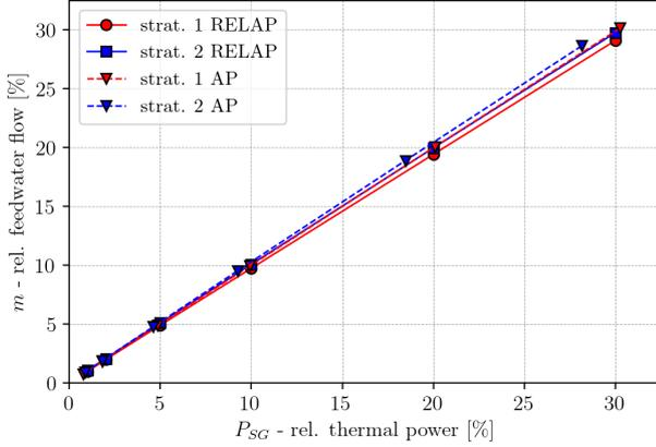
Figure 4.3 BZ OTSG relative power and feedwater flow rate trends, featuring RELAP5/Mod3.3 and Apros results.
