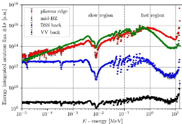
Figure 4.4 Neutron spectra at various radial planes of the equatorial breeding unit (BU) in Serpent [4].
