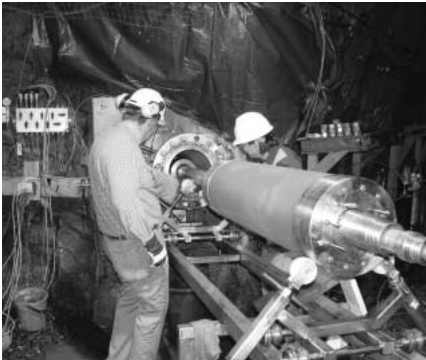
The experiment is being conducted in a part of a borehole that has been isolated from the surroundings.
