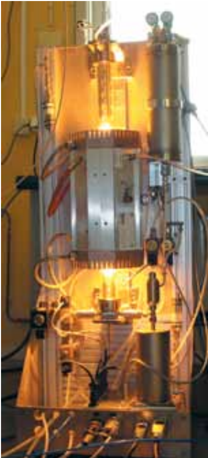
The test rig in the cell. The furnace is heated by infrared light.
